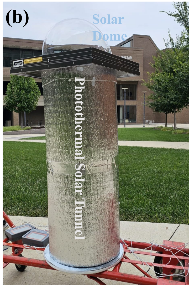
Figure 2: (a) Schematic diagram of the Photothermal Solar Tunnel (PTST) system, (b) Photograph of the solar dome connected with the PTST, and (c) The positions of thermocouples within the PTST as indicated by the red spots. The small red dots are located right on the top of each PT panel in the center and the larger red circles are located right inside the PTST at heights of 100cm, 80 cm, 60 cm, and 30 cm from the bottom of the tunnel, respectively.
