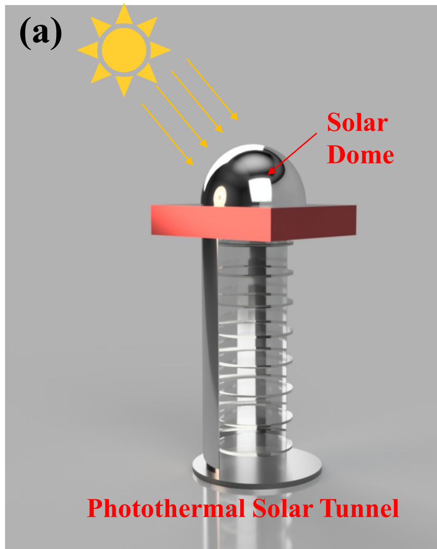
Figure 2: (a) Schematic diagram of the Photothermal Solar Tunnel (PTST) system, (b) Photograph of the solar dome connected with the PTST, and (c) The positions of thermocouples within the PTST as indicated by the red spots. The small red dots are located right on the top of each PT panel in the center and the larger red circles are located right inside the PTST at heights of 100cm, 80 cm, 60 cm, and 30 cm from the bottom of the tunnel, respectively.
