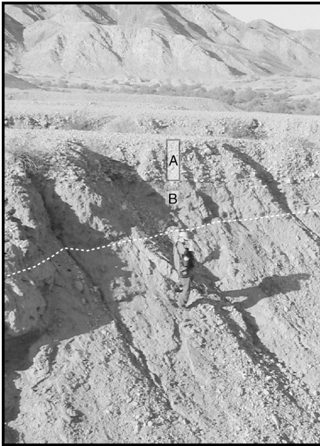
Fig. 8. Photograph showing fluvial–deltaic deposits overlain by capping gravels to form the upper surface. Location A is collection site for sample BJ2 and cosmogenic age profile for upper surface. Location B is sample site for sample BJ3, which was collected from the fluvial–deltaic deposits about 35 cm under the capping gravels. Dashed white line shows approximate bedding orientation in fluvial–deltaic deposits. Note the angular discordance of 15–17° between gravels and fluvial–deltaic deposits. View is to the northwest. Person is 2 m high for scale.
