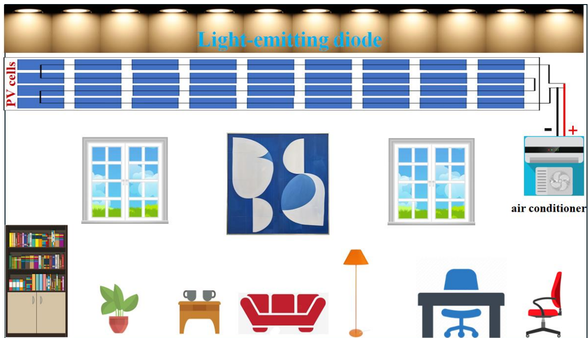
Figure 1 Indoor PV systems installed on ceilings, walls, and floors are designed to capture and convert indoor lighting into electricity. This harvested energy can be used to power various electronic appliances, such as air conditioners, reducing reliance on conventional power sources.
