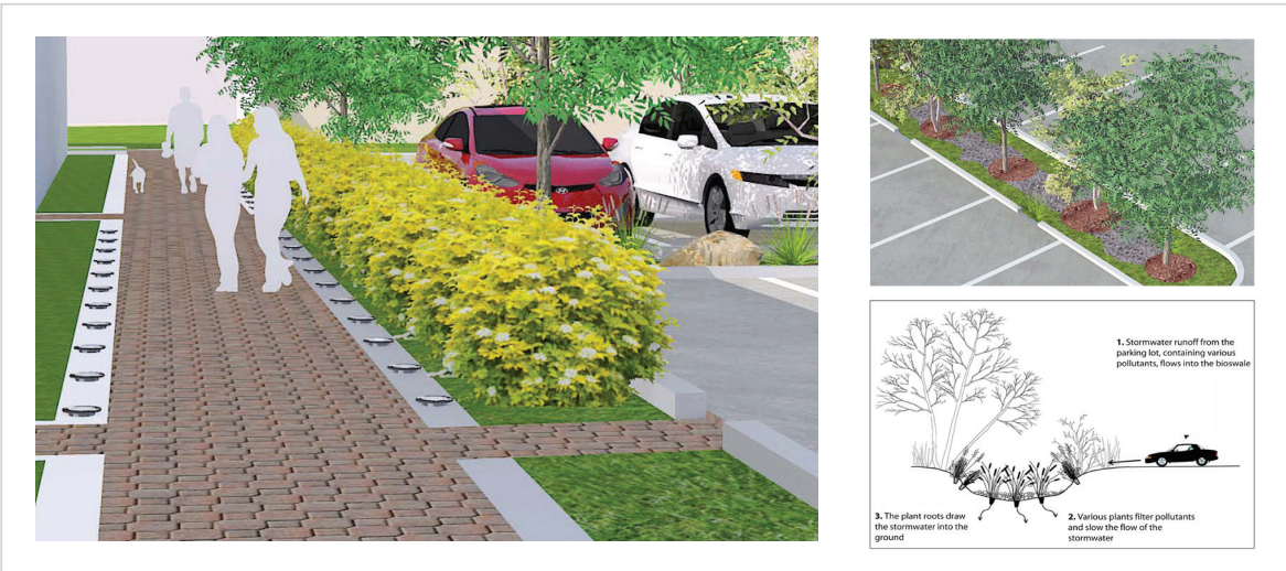
Permeable Paving, Plant Shading, and Rain Gardens in Montgomery BRT Corridor Park and Ride
