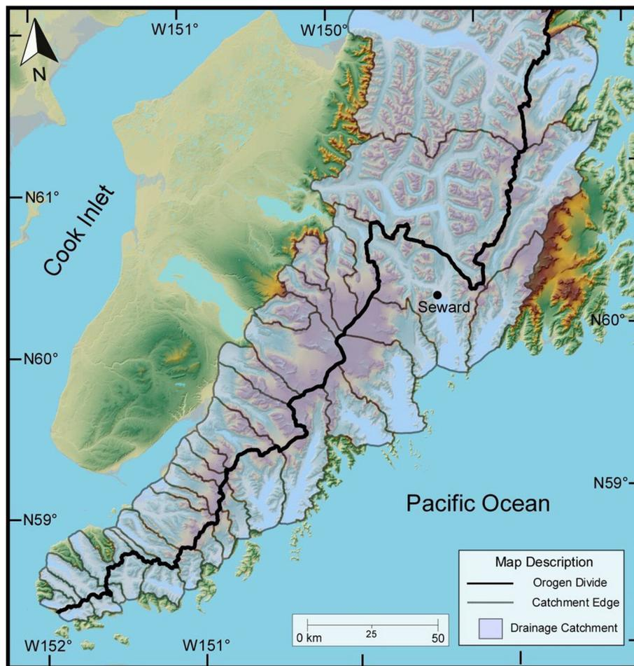
**Fig. 5.** A 300-m digital elevation model of the Kenai Peninsula showing the main drainage divide and individual catchments. The drainage divide follows the coast to the north, but steps west south of Seward. Similarly, the drainage catchments are large (1600 km<sup>2</sup>) north of Seward and substantially smaller (300 km<sup>2</sup>) to the south.
