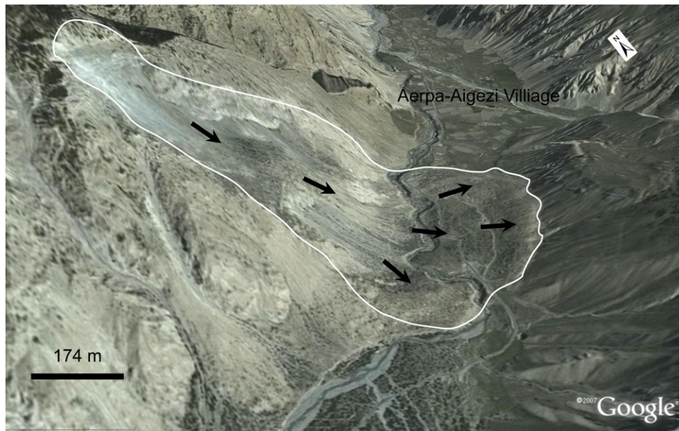
Fig. 10. Google Earth image of Aërpa Aigezi landslide showing debris accumulated on the hill opposite the landslide. Black arrows show the direction that the landslide advanced.
