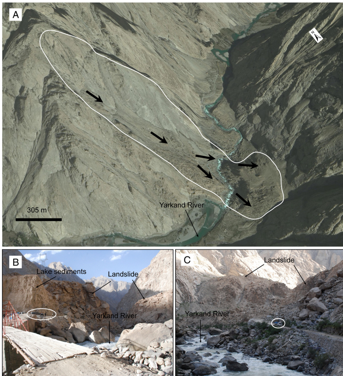
Fig. 11. Bile Jiye landslide. (A) Google Earth image of Bile Jiye landslide showing landslide debris accumulated on the opposite side of the valley. (B) View northeast looking downstream; and (C) view southwest looking upstream. Ellipses enclose people and vehicles for scale. Black arrows show the direction that the landslide advanced.
