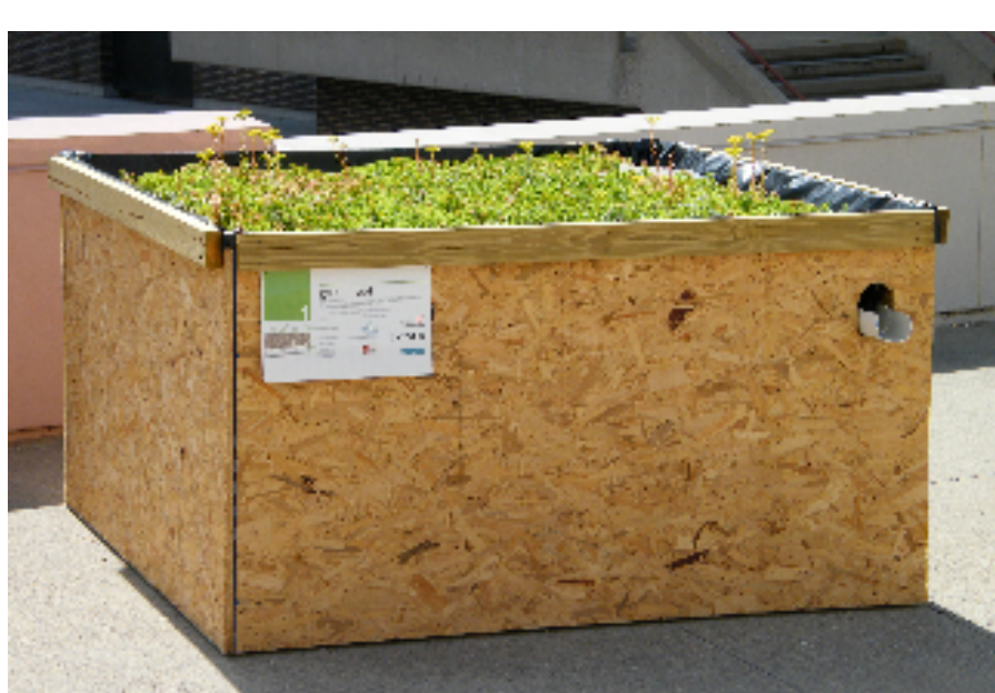
Figure 2. Prototype of experimental green roof test plots.
