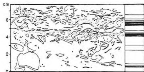
Fig.10. Sketch of a polished and acid-etched cross-section of a complex bed from the lower Wanakah at Lake Erie Shore. Fine comminuted shell debris at base of shell layers is overlain by articulated brachiopods and abundant bryozoan fragments. The column of horizontal lines on the right represents the inferred amount of time recorded by various levels within the shell bed. Closer spacing of lines indicates more time.
