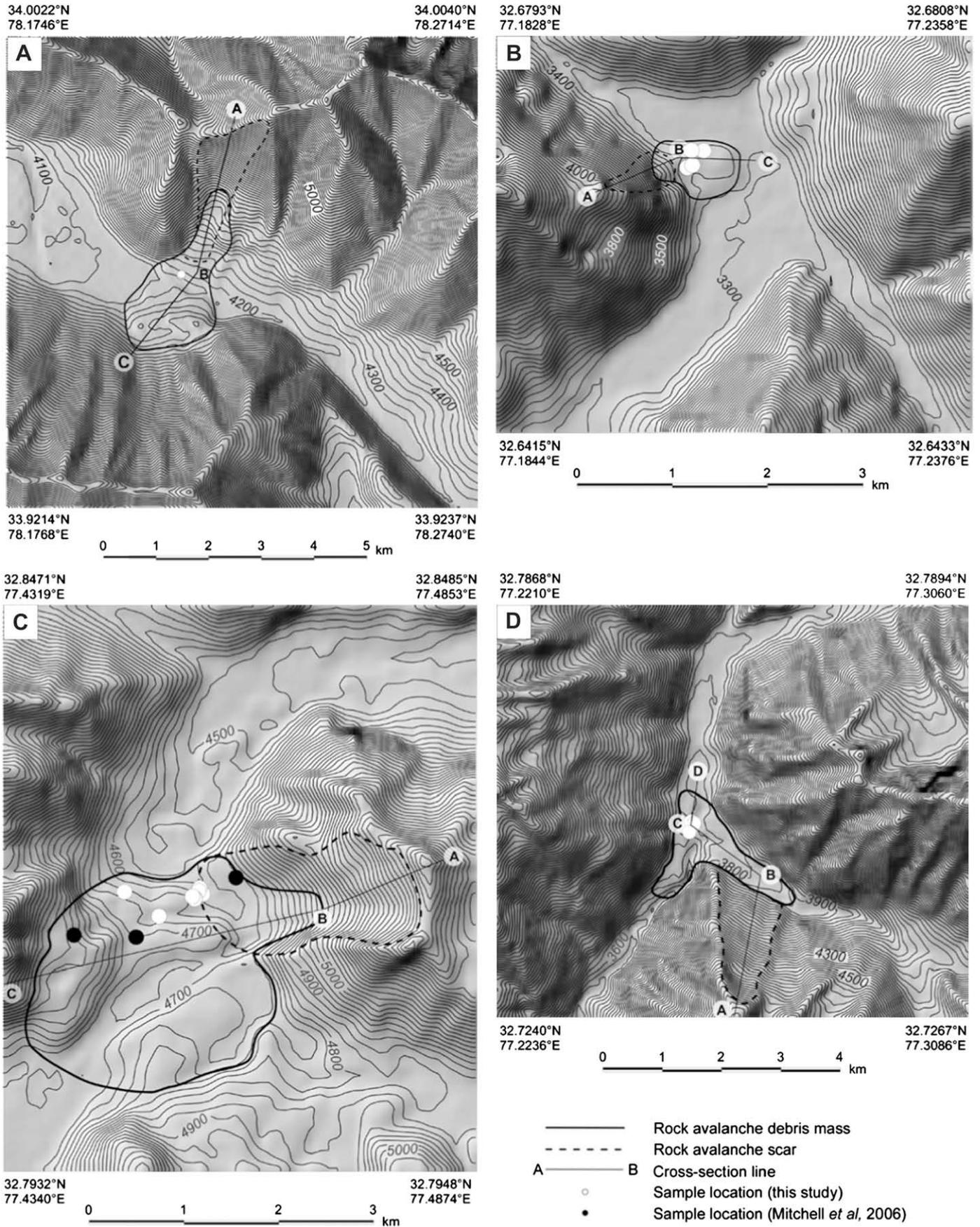
Fig. 3. DEM with contours showing the topography, deposit, scar, and sample locations (white dots) for <sup>10</sup>Be dating for the (A) Chilam, (B) Darcha, (C) Kelang Serai, and (D) Patseo landslides. Lines in A, B, C, and D show the locations of the longitudinal profiles shown in Fig. 12. The black dots in (C) are sample locations of Mitchell et al. (2007).
