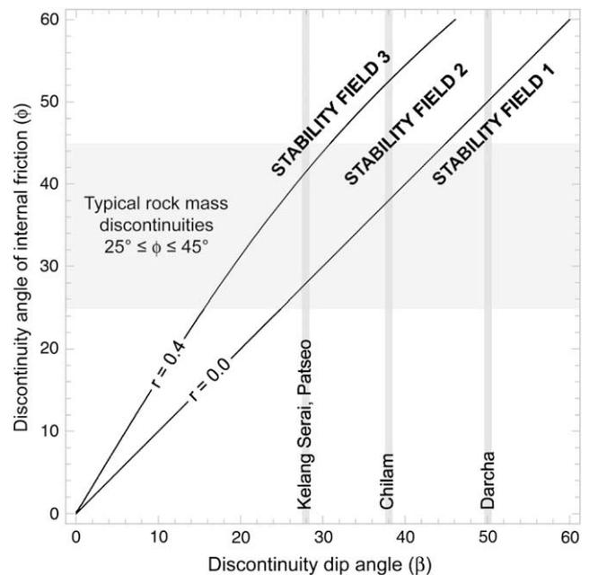
**Fig. 11.** Large landslides examined in this study plotted on idealized stability fields for frictional block sliding based on discontinuity dip and angle of internal friction. Stability field 1 is unconditionally unstable; stability field 2 can be destabilized by an increase in pore-water pressure during seismic shaking; and stability field 3 requires seismic shaking for destabilization.
