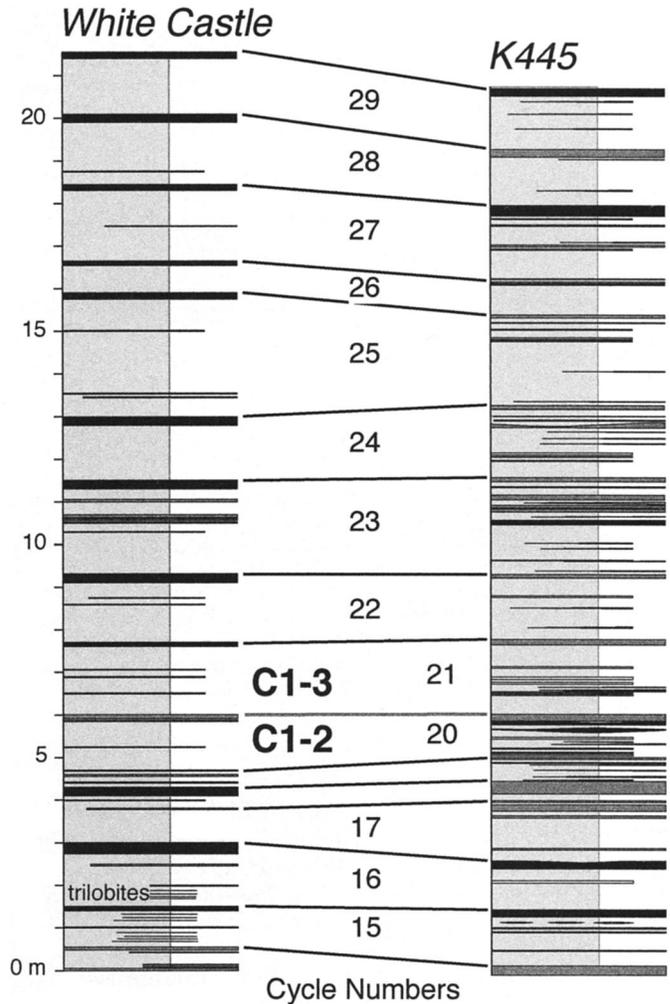
**FIGURE 8**—Final correlation of White Castle and K445 sections. Occurrence of trilobite lens at the White Castle section is equivalent to meter-scale cycle 16 of the K445 section. White Castle section spans the C1-1/C1-2 20-m cycle boundary. The fewer number of limestone beds at White Castle reflects the less intensive measurement of this section relative to K445.
